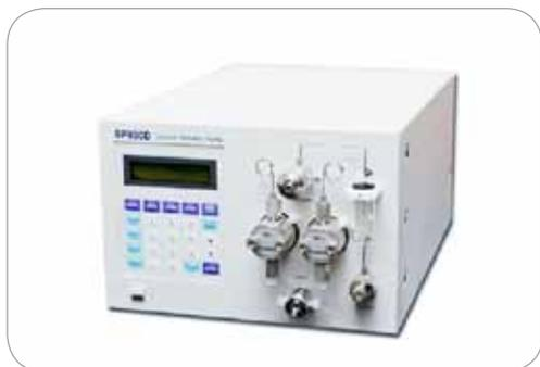
SP930D Solvent Delivery Pump is to be provided for the use of process where requires to supply accurate and precise solvent flow rate as a stand-alone unit. It can also be added to other HPLCs easily and controlled by an intuitive key pad.
